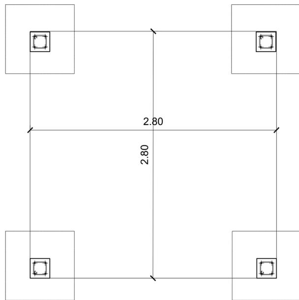
**COLUNAS E SAPATAS DA TORRE** ESCALA 1:50
